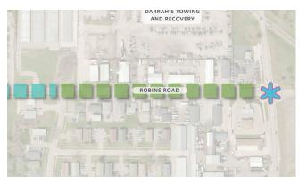
An enhanced crosswalk at the entry/exit of Robins Road will encourage the entry of a pedestrian friendly zone. There will be turn lanes that keep traffic moving smoothly and give easy access to businesses. On-street parallel parking is proposed on the west side of the street with permeable pavers.
